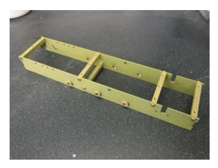
In the pictures I have taken the time to find an etch primer that works well with ferrous and non ferrous metals to accommodate both brass and steel parts. This primer is a 'wash primer' and has very little build so will not affect the alignment of the frame setup with an inadvertently uneven application of paint. Once happy with the frames it will be time to paint them in the final colour before assembly.
