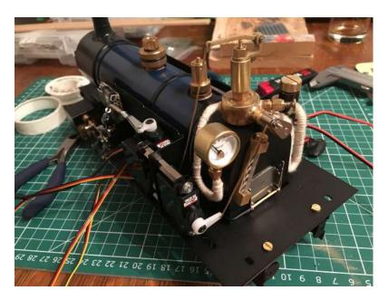
R/c regulator, forward/reverse gear, dampener and whistle. Cleverly made linkages that operate from three servos.
