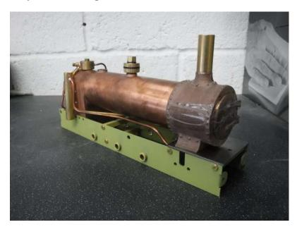
So with the boiler confirmed to be fitting on the frames, I painted them I n a satin 2k solid black and assembled the chassis. The theory being that if the chassis is set up correctly 'as per instructions' it should work. I do pride myself on getting a chassis running well so I spend a lot of time measuring and remeasuring all events and making good where required.
