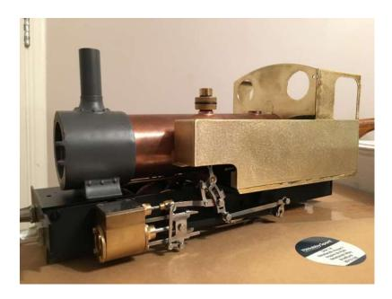
So with the body complete it was time to paint the boiler wrapper and fit it to the chassis for the last time and get going with all of the r/c equipment. I really wanted to steam the loco anyway!
