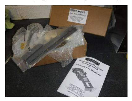
So to begin with we need to start with something, something in the form of main frames, spacers and a little extra that Roundhouse supplied also. Joep makes mention to omitting of one chassis spacer that is towards the rear of the frame set up, this is to accommodate the firebox between the frames as it sits deep towards the bottom of the frame set.
